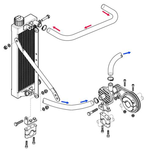
After filling the circuit (pure water only), provide for proper air vent.
