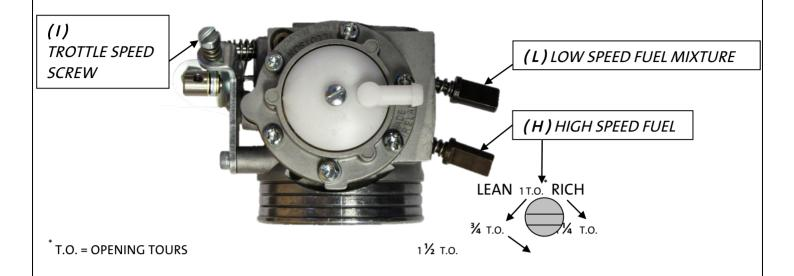
The recommended setting of the carburetor screws, after run-in, is the following:
